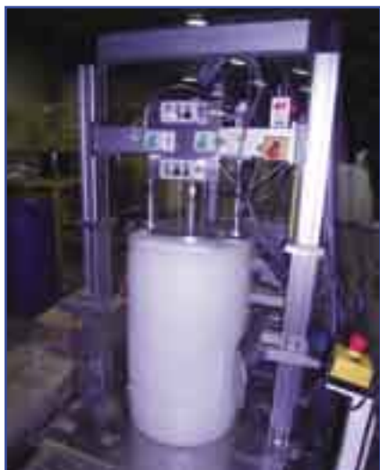
First PE drum being leak tested in Melbourne.
